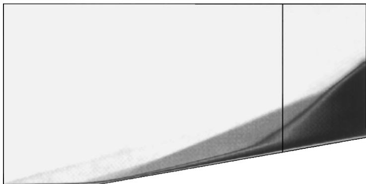
FIG. 23. Temperature for extended domain: M = 4.0 hydrogen/air 10^\circ viscous ramp, 128 \times 156 grid. Temperature range, 1200–3500 K. Solid line in the computational domain indicates original outflow boundary.
